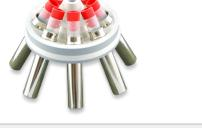
Angular 8 x 10/15 mL./ Max: 6000 Rpm./ FCR Max: 4226 xg / 30°. Tubos Falcon.                           |
