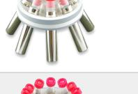
Angular 8 x 10/15 mL. / Max: 6000 Rpm. / FCR Max: 4226 xg / 30°. Tubos Falcon.                           |
